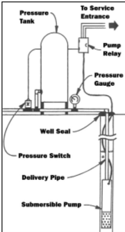
**Figure 1:** Components of the "demand" type system.
