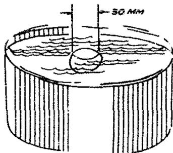
FIGURE 7. THE STRENGTH OF A LYE SOLUTION CAN BE TESTED BY FLOATING AN EGG IN IT. A SOLUTION OF THE CORRECT STRENGTH WILL RAISE PART OF THE EGG OUT OF THE WATER, FORMING AN OVAL ABOUT 30 MM LONG AT THE WATER'S SURFACE.
