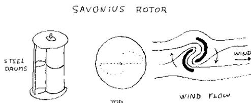
Our present Savonius rotor is a variation of the Brace Research Institute's design<sup>5</sup>, using 55-gallon steel drums cut lengthwise and welded into two off-set cup-shaped blades. Bearings at top and bottom in a guyed wooden frame complete the rotor. (A few hints: Use 4x4 inch lumber for the frame; balance the rotor carefully; and wire the turnbuckles when tight as they can vibrate loose.)
