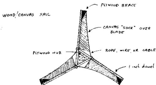
of the tower, probably at a slight dihedral angle for added stability. Higher gearing will be necessary (about 20:1), but we feel that a larger blade diameter (15 feet), simple construction, and less centrifugal stress will make the test worthwhile.
