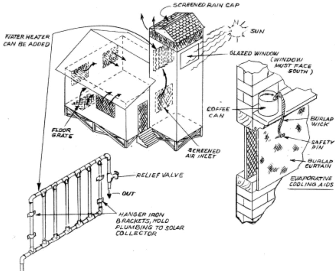
water heating system, no matter how it's fueled. So, not including a relatively inexpensive pressure relief valve would just be like begging for trouble here. Also, while possibly unneeded in many tropical areas, in more temperate climates you'll need a means of draining and bypassing this system during the winter months.
