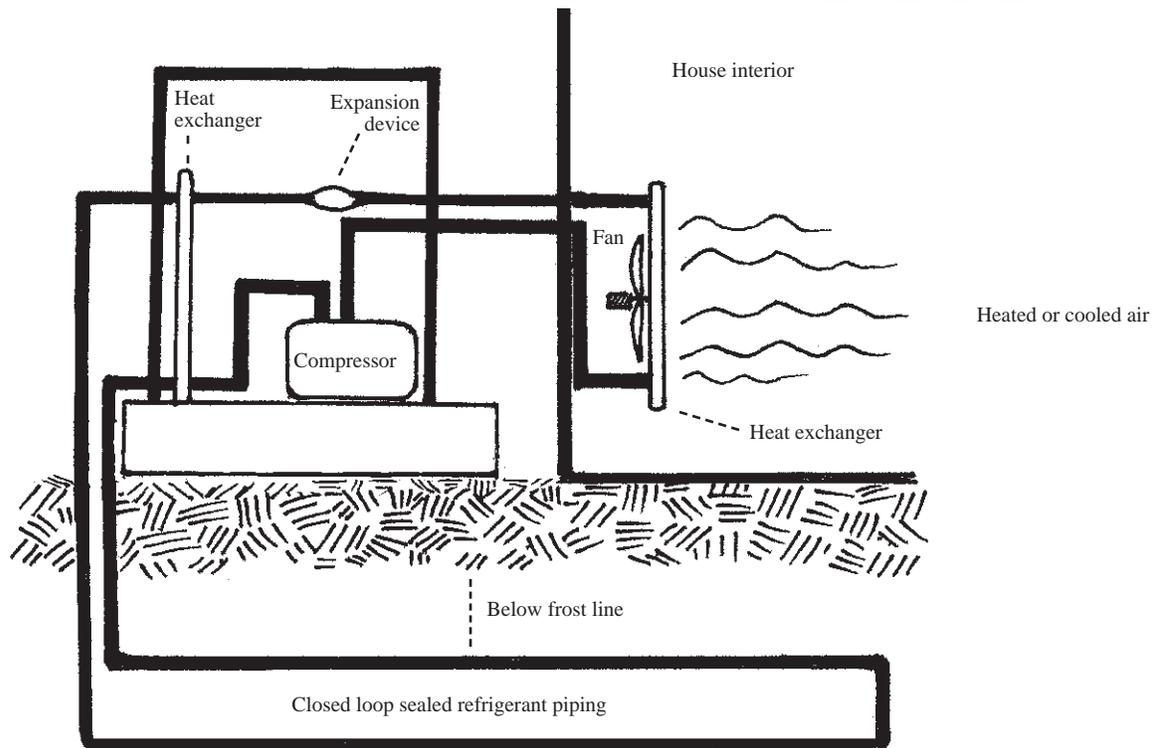
*Components of a GSHP. Underground piping may be vertical in a borehole, horizontal in a narrow trench, or in the form of a continuous coil in a wide trench. Piping may be above or below the water table. Compressor and expander can be in the building being served or in a shelter outside.*
