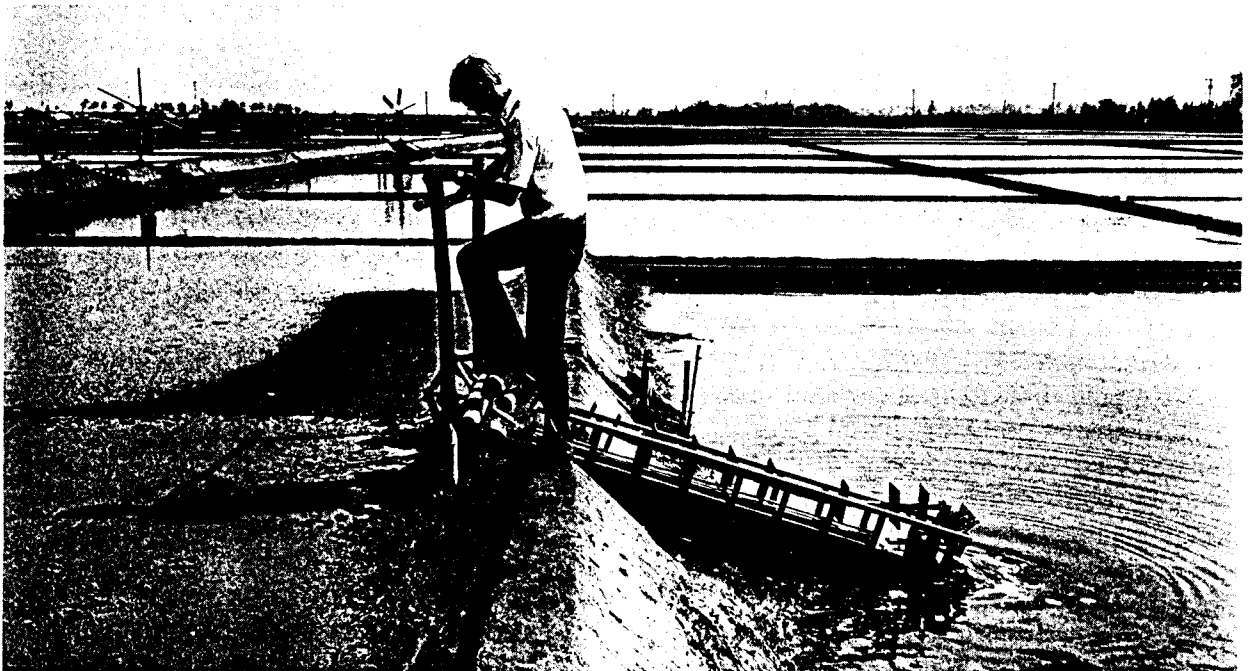
Figure 2-19 Chinese wooden water pump used for raising sea water into salt-evaporation beds
