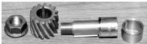
mate with the alternator shaft. On the other end, I machined an outside thread to accommodate the bolt that holds the gear in place. This part was 3½ inches long. I broached the keyway into the machined shaft and slowly removed material from the female end until the overall length made for perfect alignment of the gears.
