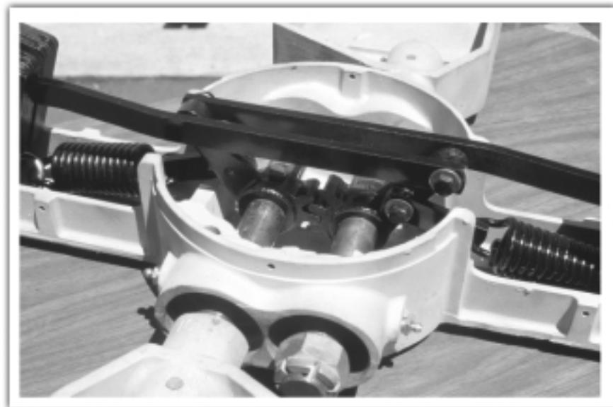
(Above) At rated speed, the governor's weights arc outward, pulling the gears and prop shafts into rotation, preventing rotor overspeed.
