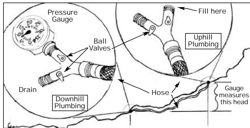
mate the gauge with the plastic Y-fitting. This will depend on the type and size of thread on the gauge you find. If you take all the parts to a hardware store, you can usually figure out what you need or get some help.
