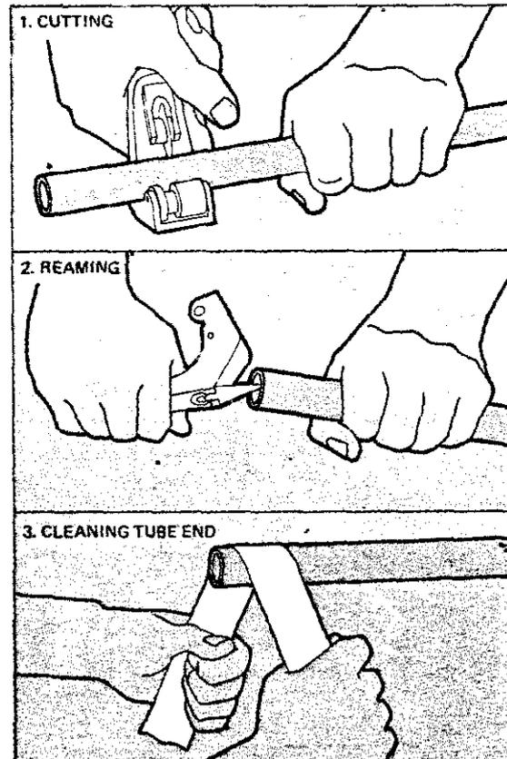
Cut pipe to length using a tubing-cutter (1) or a fine hacksaw blade. Make sure the cut is square and the pipe remains round and true. Cutting with a hacksaw blade leaves rough edges on the inside and outside of the pipe, while a tubing cutter leaves rough edges on the inside of the pipe. Remove burrs on the outside of the pipe with a smooth file or sandpaper and on inside with a reamer (2) or rattail file. Clean the end of pipe with steel wool or a strip of sandpaper (3).
