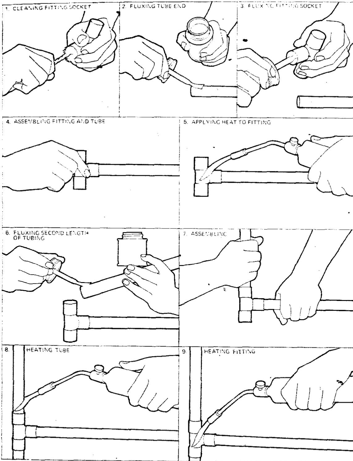
Clean the inside of the fitting with a wire brush. A thorough cleaning is absolutely necessary because a "sweat" joint relies on capillary action and any dirt, grease, or surface oxidation on the pipe or the fitting will hinder the joining action. Because the pipe should fit tightly into the fitting, do not remove too much metal when sanding or the capillary space will be enlarged and the joint weakened.
