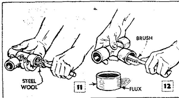
of the fitting) must be cleaned thoroughly with fine steel wool or emery cloth, rubbing the metal as in Fig. 11 until it is bright. Wipe the tubing clean, then apply a thin film of soldering flux, Fig. 12. Push the tubing into the fitting as far as it will go, then rotate it a few times to assure even distribution of the flux.
