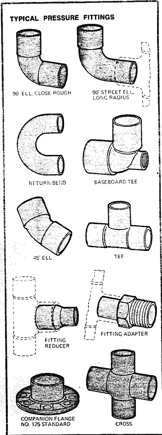
Copper piping is light and extremely durable, requires no threading of the ends to join it, comes in varying diameters, wall thicknesses and degrees of hardness, and is suitable for both hot and cold-water systems. To join copper piping, there are many types of fittings to cover every part of the plumbing layout. A number of common fittings are shown at the left.
