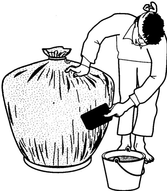
3. When full, tie the top sacking and form into a jar shape by tapping with a block of wood. Spray with water before plastering.
