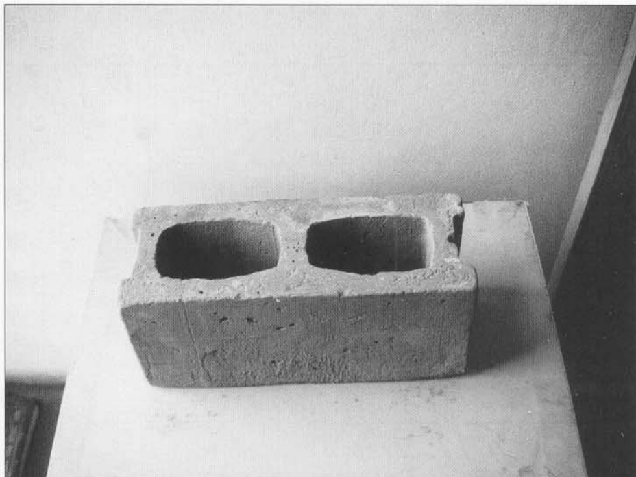
Fig.1: Hollow building block of "Red Mud Pozzolanic Cement"
